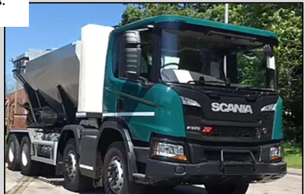
DURALight low weight, high strength design allows a full 8m 3 payload within the 32 tonne legal GVW
