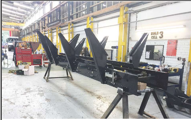
STRENX 700 Subframe and bin supports for weight saving and increased strength
