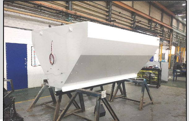
HARDOX 450 Aggregate bins for superior wear resistance, strength and service life
